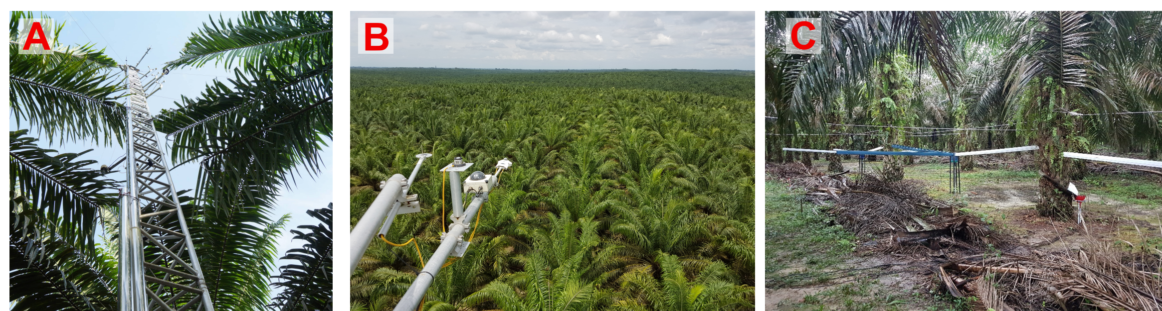
Fig. 1: Climate measurement tower (A), top-of-tower view (B), below-canopy structure and throughfall measurements (C).
